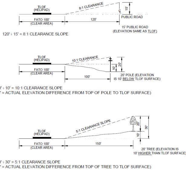
NOTE : 1. OBSTACLE CLEARANCE SLOPE IS CALCULATED ON DISTANCE OF OBSTACLE FROM THE FATO EDGE.
