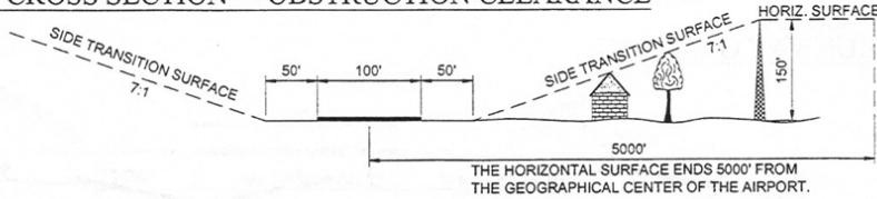
**§154.31.5 Design and Layout Requirements for a Tall Structure Near a Heliport**
